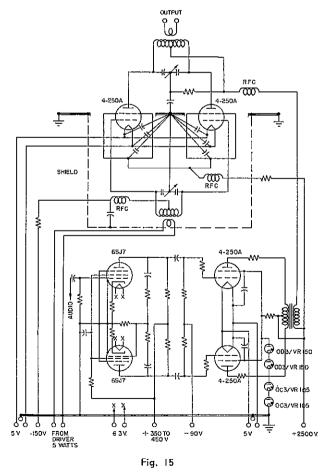
Typical high-level-modulated r-f amplifier circuit with modulator and driver stages, 1000 watts input.
