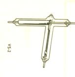
A single pole, double throw switch with contacts in high vacuum for high voltage switching. Contact spacing .015". Switch will handle r-f potentials as high as 20 Kv. In DC switching will handle approximately 1.5 amps. at 5 Kv.
