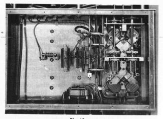
Fig 12 Underside of push-pull multi-band r-f amplifier employing 4-250A tetrodes. Designed and built by C. F. Bane (W6WB)<sup>6</sup>.
