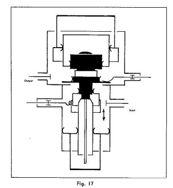
Schematic cavity section of 1250 Mc., amplifier employing 4X150G tetrode.
