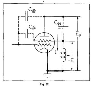
Tetrode characteristics involved in feedback circuit.
