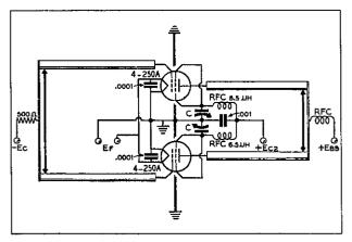
Screen-tuning neutralization circuit for use above 45 Mc. C — Approximately 100µµfd. per section, maximum.
