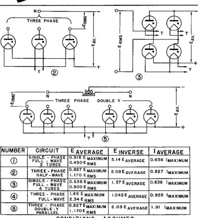
GONDITIONS ASSUMED SINE WAVE SUPPLY, BALANCED PHASE VOLTAGES, ZERO TUBE DROP, PURE RESISTANCE LOAD, NO FILTER USED.
