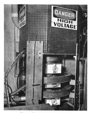
Fig. 8-The 5-kw klystron on test.
