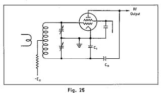
Push-pull grid neutralization, basic circuit.
