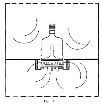
DO NOT SUB-MOUNT A METAL BASE SHELL TUBE. Base cooling is prevented and no improvement in shielding results.
