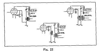
Basic high-level-modulating circuits for tetrodes.
