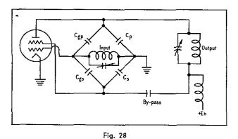
Single-ended plate neutralization showing capacitance bridge circuit present.
