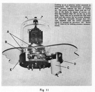
Eimac 4-400A/4000 Air System Socket providing balanced tube cooling by a single stream of air.
