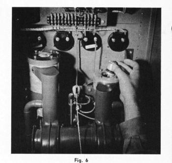
Experimental 950 Mc. doubler final and tripler driver employing 4X150A tetrodes. Designed and built by Eitel-McCullough Laboratories.
