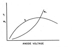
Fig. 5-Power output and efficiency versus anode voltage.
