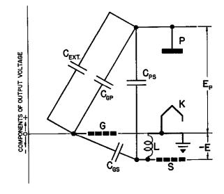
Fig. 31 Components of output voltage of a tetrode when neutralized by added sories scroen-lead capacitance.
