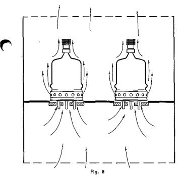
4-125A mounting providing cooling, shielding and isolation of output and input compartments.
