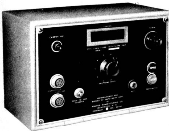
Figure 2-27. Radiophone Unit Navy Type -23500, Front View, Showing Controls
