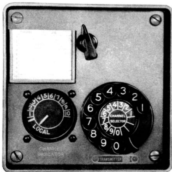
Figure 2-21. Remote Channel Selector Navy Type —23445, Front View, Showing Controls
