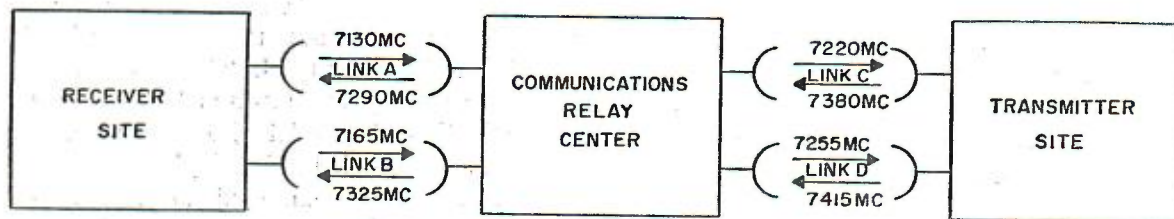
Figure 7-12. Typical Intersite Microwave Radio Links.
